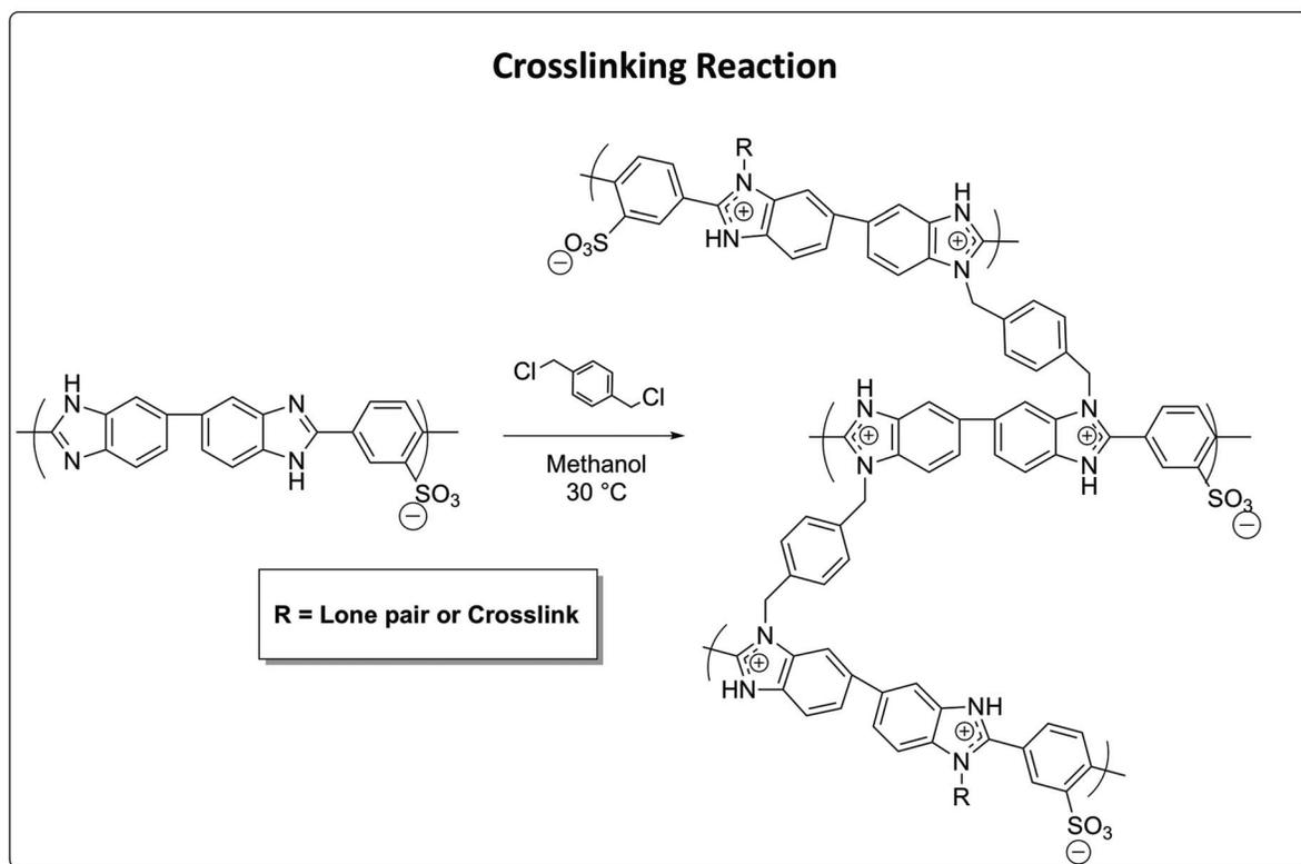
**Scheme 1.** Polymerization of s-PBI in PPA and membrane crosslinking modification reaction.
