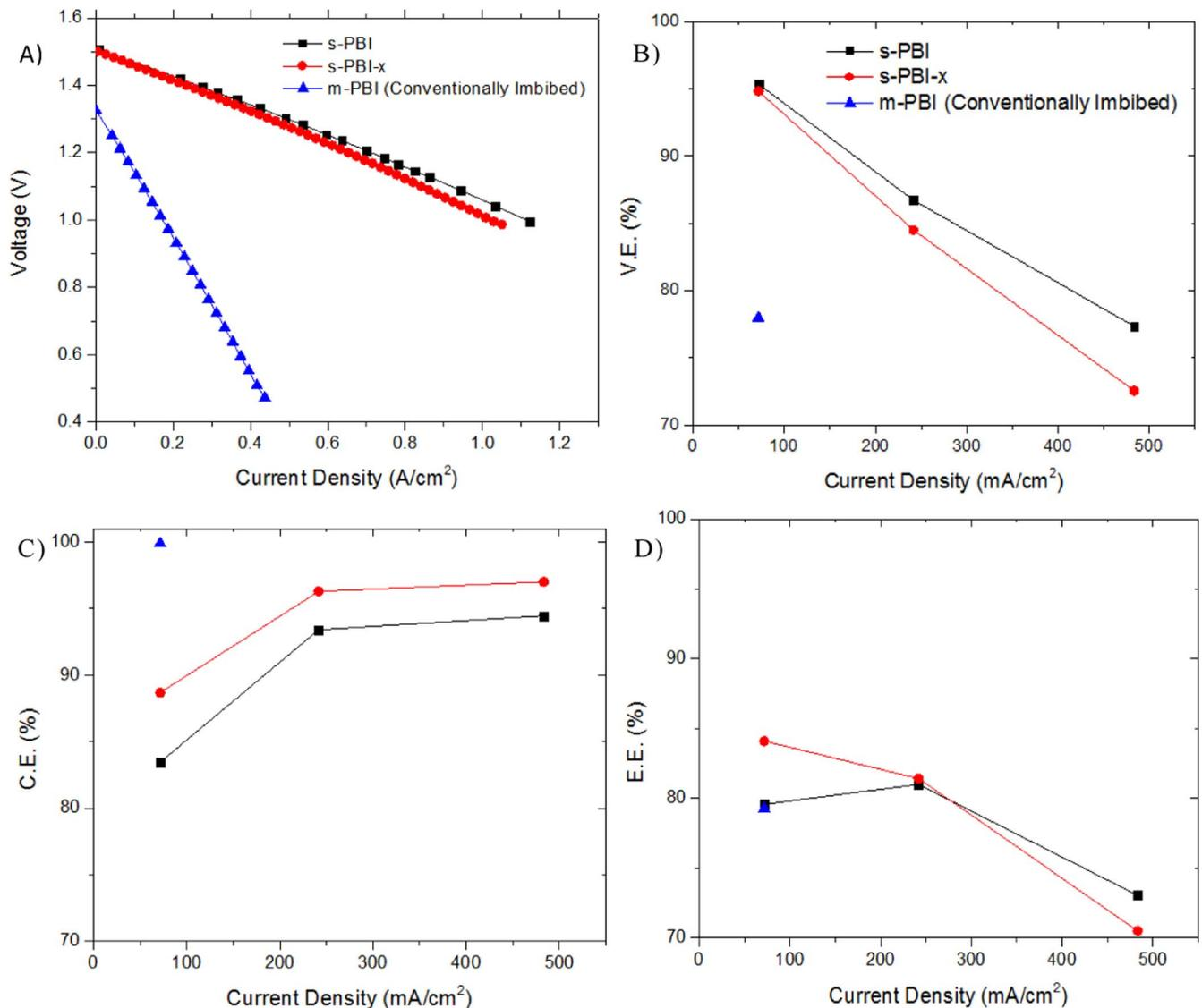
**Figure 3.** A) Polarization curves with 80% state-of-charge electrolyte, and cycling efficiencies; B) voltage efficiencies, C) coulombic efficiencies, and D) energy efficiencies of VRB cells that were otherwise identical but utilized with three different membranes: s-PBI, s-PBI-x, and m-PBI (conventionally imbedded).
