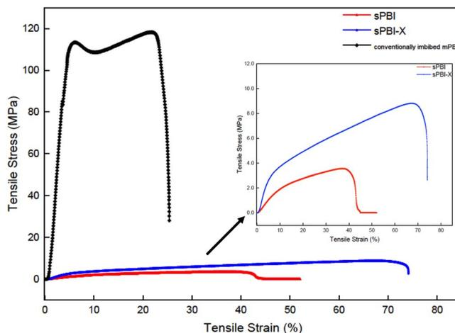
**Figure 2.** Stress-strain curves for water imbibed s-PBI ( $80.4 \pm 0.7\%$  H<sub>2</sub>O), s-PBI-x ( $76.8 \pm 0.3\%$  H<sub>2</sub>O) and conventional m-PBI ( $16.3 \pm 2.9\%$  H<sub>2</sub>O) membranes.
