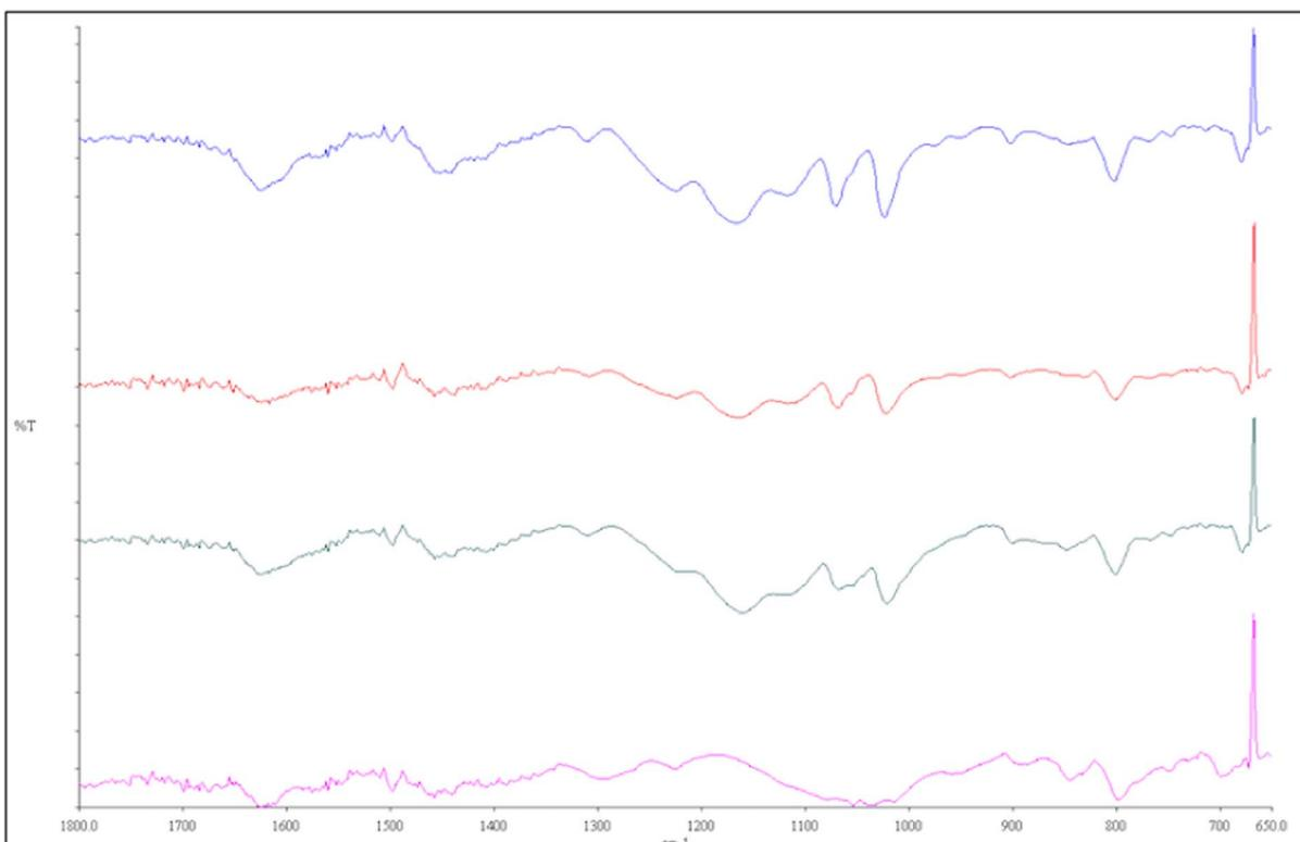
**Figure 1.** ATR-FTIR spectra of a) s-PBI membrane before cell testing; b) s-PBI membrane after cell testing; c) s-PBI-x membrane before cell testing; b) s-PBI-x membrane after cell testing. All membranes were examined after treatment overnight at 120°C.
