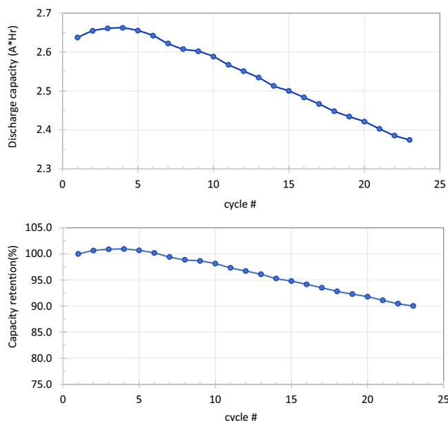
**Figure 4.** Discharge capacities and and capacity retention of VRB with s-PBI-x membrane in 23 cycles.
