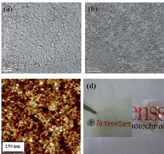
**Fig. 4** TEM image of TiO<sub>2</sub>-PGMA composites (a) 35 wt%, (b) 55 wt%; (c) AFM image of TiO<sub>2</sub>-PGMA (55 wt%); (d) photograph of coating of TiO<sub>2</sub>-PGMA (55 wt%) on glass slides (with a thickness of 20 μm) and transparent self-standing film.
