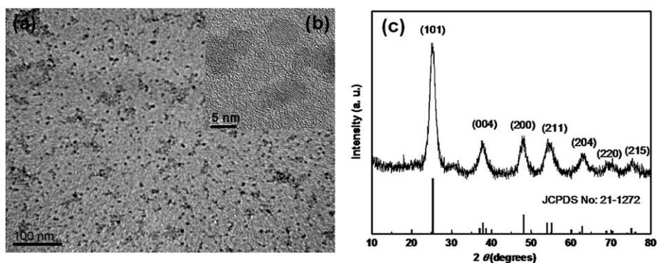
Fig. 1 (a) TEM, (b) HRTEM image, (c) XRD pattern of as-synthesized TiO<sub>2</sub> nanoparticles.
