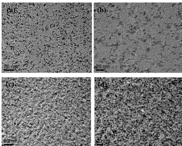
Fig. 7 TEM images of TiO<sub>2</sub>-epoxy nanocomposite at low and high magnification: (a, b) 10 wt% TiO<sub>2</sub> loading; (c, d) 30 wt% TiO<sub>2</sub> loading.
