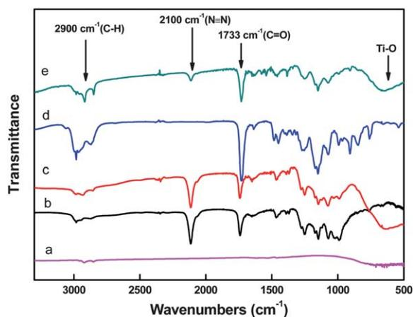
Fig. 2 FTIR spectra of (a) as-synthesized TiO<sub>2</sub>, (b) phosphate-azide ligand, (c) TiO<sub>2</sub> treated with phosphate ligand, (d) alkyne-terminated PGMA, (e) TiO<sub>2</sub>-click-PGMA.
