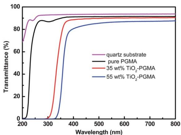
Fig. 6 Transmittance spectra of TiO<sub>2</sub>-PGMA composites with thickness about 20  $\mu\text{m}$ .
