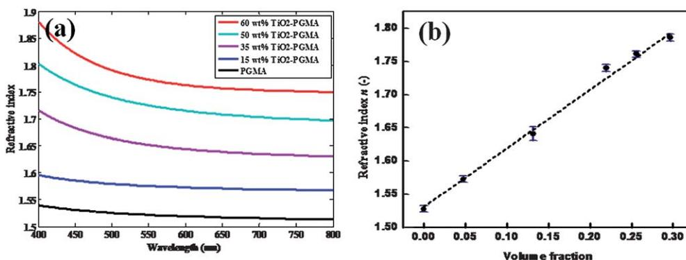
**Fig. 5** (a) Refractive index dispersion of TiO<sub>2</sub>-PGMA composite and neat PGMA; (b) plot of refractive index of TiO<sub>2</sub>-PGMA composite dependence on TiO<sub>2</sub> volume fraction.
