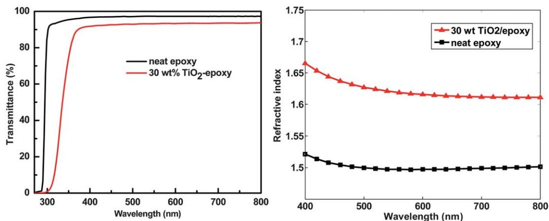
Fig. 8 Transmittance spectra and refractive index dispersion of neat epoxy and TiO<sub>2</sub>-epoxy nanocomposites.
