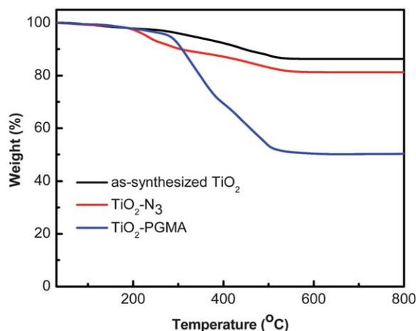
Fig. 3 TGA curves for the as-synthesized TiO<sub>2</sub>, TiO<sub>2</sub>-phosphate-azide, and TiO<sub>2</sub>-click-PGMA.
