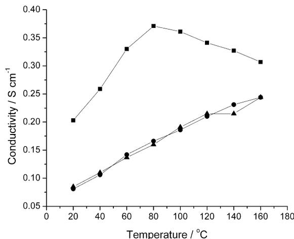
Fig. 4 Effects of temperature on ionic conductivity for PA-doped *para*-PBI membrane (squares, 1st run; circles, 2nd run; triangles, 3rd run).
