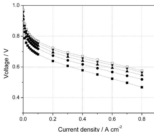
Fig. 9 Polarisation curves of *para*-PBI membrane based fuel cells with hydrogen (415 mL min<sup>-1</sup>)/air (1,655 mL min<sup>-1</sup>) at 160 °C under different gas pressure. (Filled squares, 1 atm; filled circles, 1.5 atm; filled triangles, 2 atm; filled stars, 2.5 atm; and unfilled squares, 3 atm; absolute pressures).
