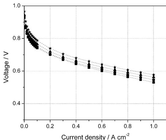
Fig. 8 Polarisation curves of *para*-PBI membrane based fuel cells with hydrogen ( $\lambda = 1.2$ )/oxygen ( $\lambda = 2.00$ ) at different temperatures under ambient pressure by constant stoic mode. (Squares: 120 °C, circles: 140 °C, triangles: 160 °C and stars: 180 °C).
