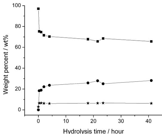
Fig. 3 The change in phosphoric acid doped *para*-PBI membrane composition (squares, phosphoric acid; circles, water; stars, *para*-PBI) with time when hydrolysed at 25 °C, 40% RH.
