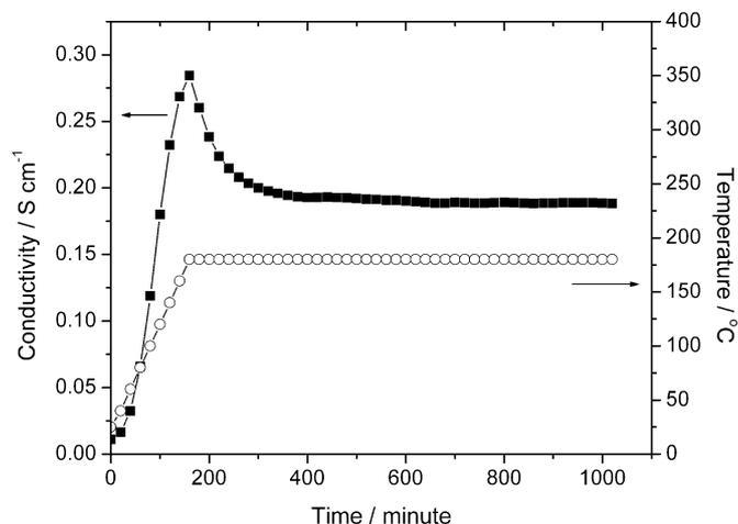
Fig. 5 Long-term conductivity measurements at 180 °C for *para*-PBI/PA membrane.
