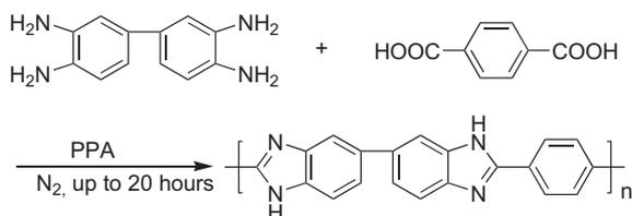
Fig. 1 Synthetic scheme for the synthesis of *para*-PBI in polyphosphoric acid (PPA).
