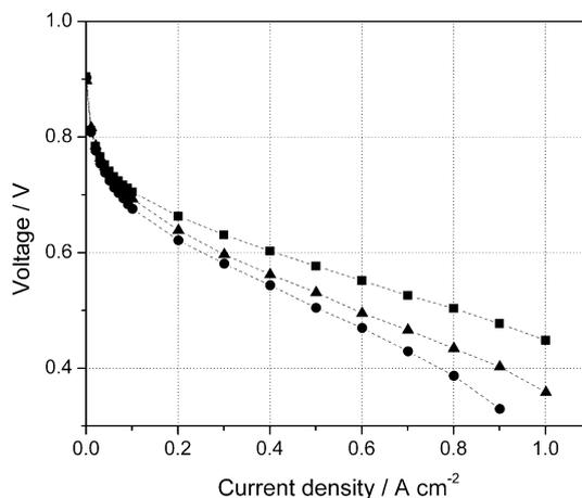
Fig. 7 Polarisation curves of *para*-PBI membrane based fuel cells with hydrogen/air and reformate/air at 180 °C under ambient pressure. [Squares: hydrogen/air, triangles: (reformate composition I, H<sub>2</sub> 70%, CO 1%, CO<sub>2</sub> balance)/air and circles: (reformate composition II, H<sub>2</sub> 35.8%, CO 0.2%, CO<sub>2</sub> 11.9%, N<sub>2</sub> balance)/air by constant stoic mode, fuel ( $\lambda = 1.2$ )/air ( $\lambda = 2.0$ )].
