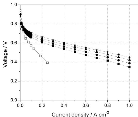
Fig. 6 Polarisation curves *para*-PBI membrane based fuel cells with hydrogen ( $\lambda = 1.2$ )/air ( $\lambda = 2.00$ ) at different temperatures and at ambient pressure (1 atm, absolute) by constant stoic mode. [Squares: 120 °C, circles: 140 °C, triangles: 160 °C and stars: 180 °C]. Open squares are data from reference [2] on PA doped m-PBI at 150 °C.
