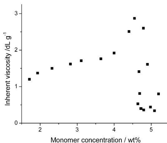
Fig. 2 Effect of monomer concentration on the *para*-PBI inherent viscosity (I.V.) at a polymerisation temperature of 195 °C.
