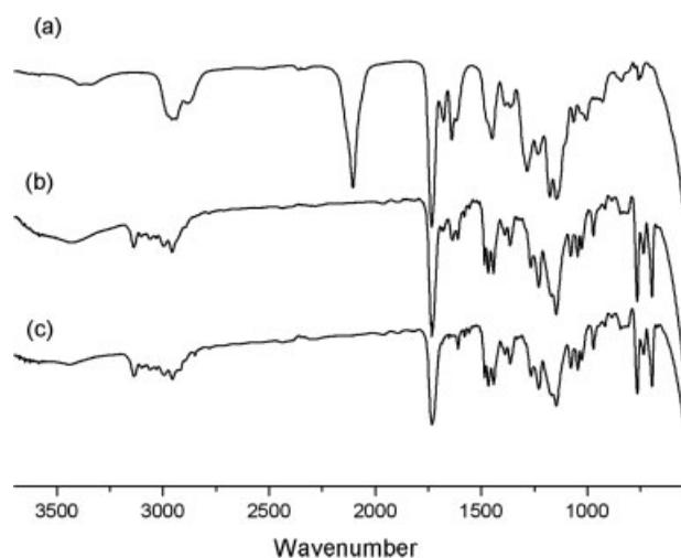
**Figure 5.** IR spectra of (a) polyAzMA, (b) polyTriazoleMA (postfunctionalization route) and (c) polyTriazoleMA (prefunctionalization route).
