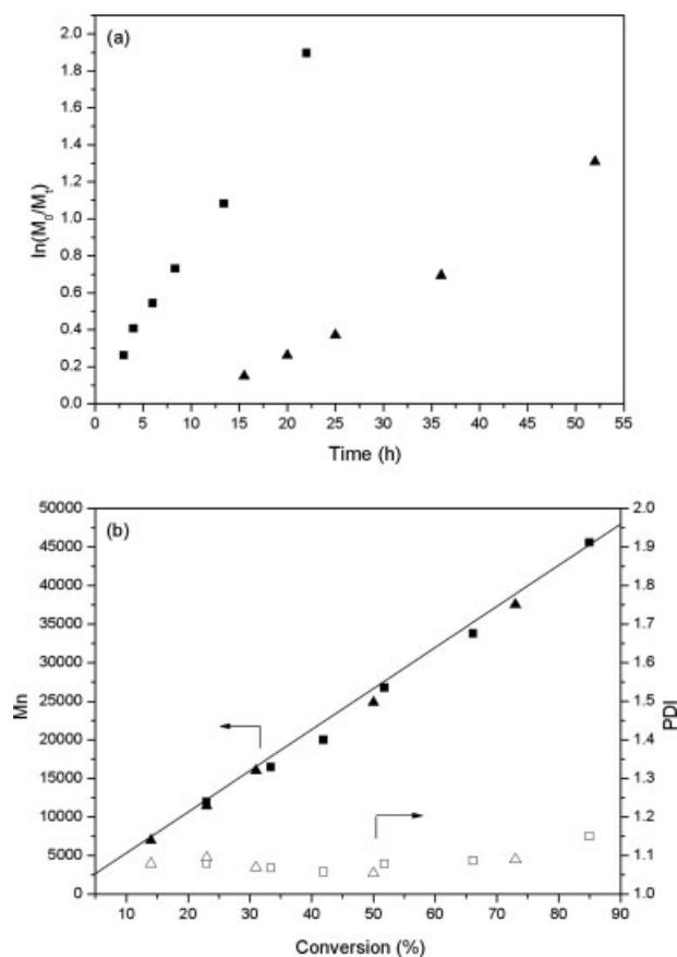
**Figure 3.** (a) Kinetic plots and (b) dependence of the molecular weight and polydispersity on the conversion for the RAFT polymerization of AzMA ( $[\text{AzMA}]:[\text{CPDN}]:[\text{V-70}] = 344:1:0.1$ ): (squares)  $40\text{ }^\circ\text{C}$  and (triangles)  $30\text{ }^\circ\text{C}$ .
