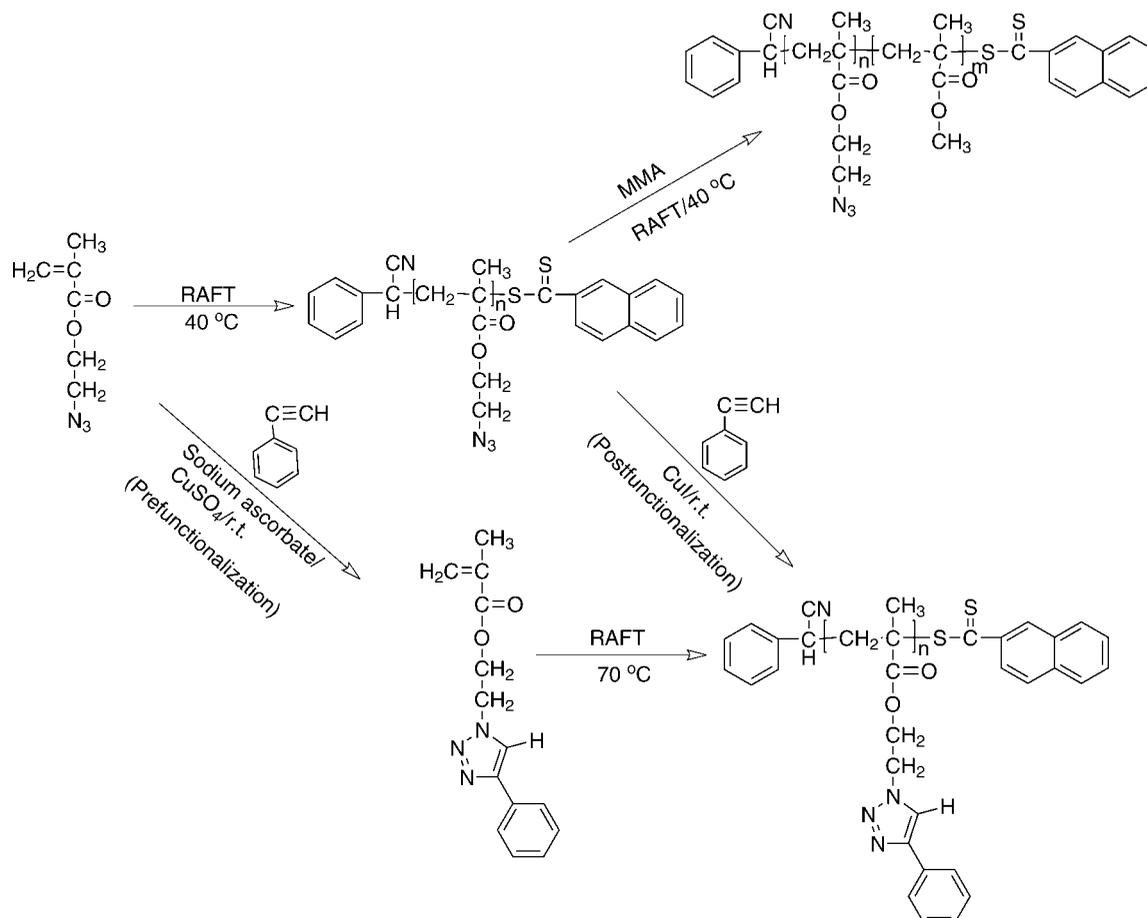
**Scheme 2.** Preparation of polyAzMA and polyAzMA derivatives by combining RAFT polymerization and click chemistry.
