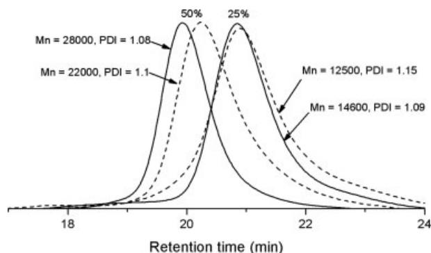
**Figure 7.** GPC traces for polyTriazoleMAs (dash lines) and their precursory polyAzMAs (solid lines) prepared at 25% and 50% conversions for 40 °C polymerizations.
