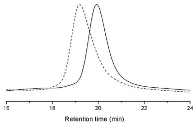
**Figure 4.** GPC traces for (solid line) polyAzMA ( $M_n = 21,500$ ; PDI = 1.08) and (dashed line) polyAzMA-*b*-poly(methyl methacrylate) ( $M_n = 30,000$ ; PDI = 1.12).
