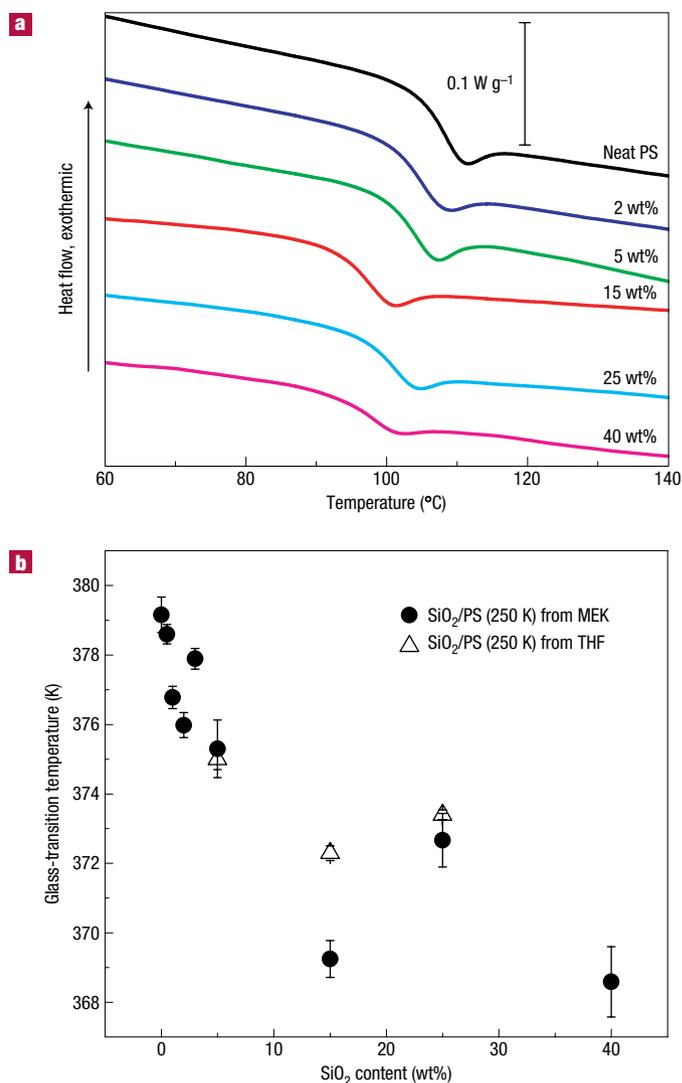
**Figure 2** The glass-transition behaviour of  $\text{SiO}_2/\text{PS}$  nanocomposites.
