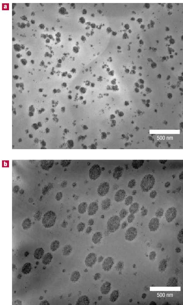
**Figure 5** The effect of solvent on the agglomeration of nanoparticles. **a, b**, TEM images of 15 wt% SiO<sub>2</sub>/PS nanocomposites prepared by MEK (**a**) and THF (**b**). Although the extents of agglomeration are quite different in the two cases, we note that their  $T_g$  shifts can be rationalized by calculating the  $h_z^{***}$  values. These results emphasize that particle size is a secondary concern in this context.
