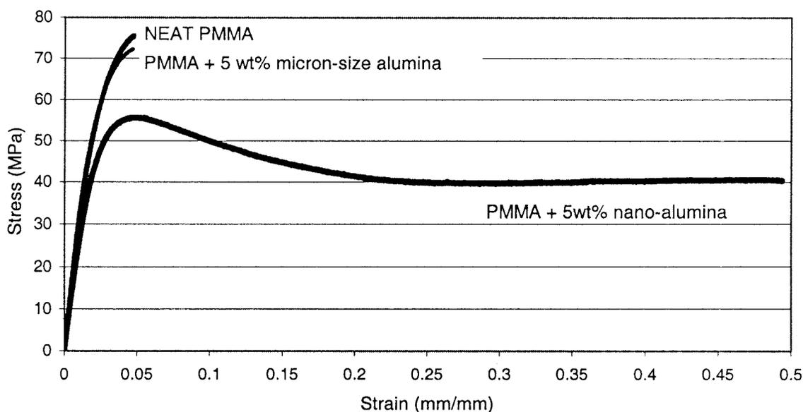
Fig. 2. Stress versus strain curves for 1 mm min<sup>-1</sup> strain rate. Unlike either the neat or micron-filled polymer, the nano-alumina filled PMMA clearly shows a yield point followed by a constant stress, increasing strain region.
