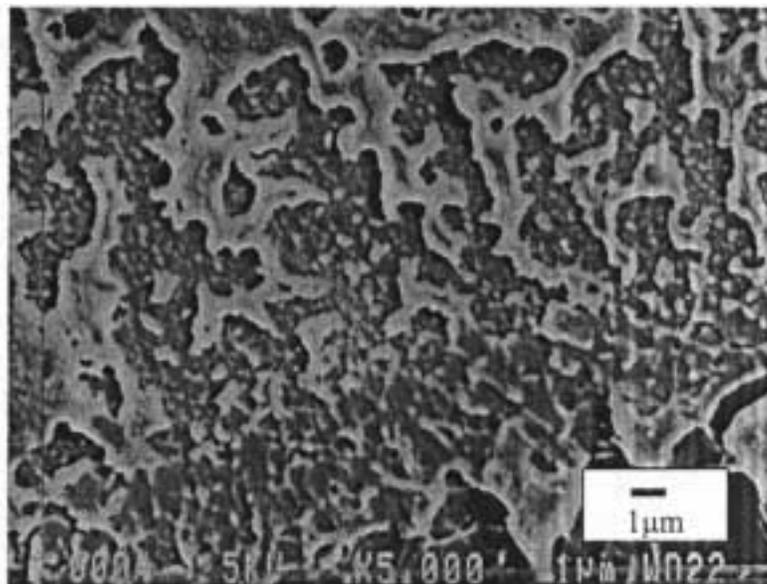
Fig. 7. Low resolution SEM micrograph of heavily yielded (40% elongation) PMMA/nano-alumina composite (5 wt%) showing fast fracture behavior initiating at a defect.
