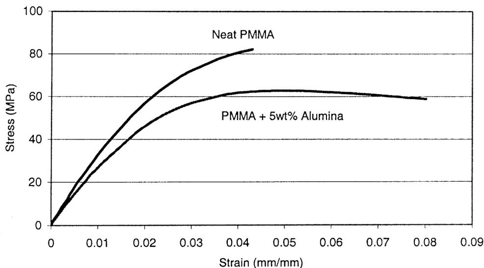
Fig. 3. Stress versus strain curve showing yield behavior in the 5 wt% nano-alumina sample at higher strain rate ( $10 \text{ mm min}^{-1}$ ).
