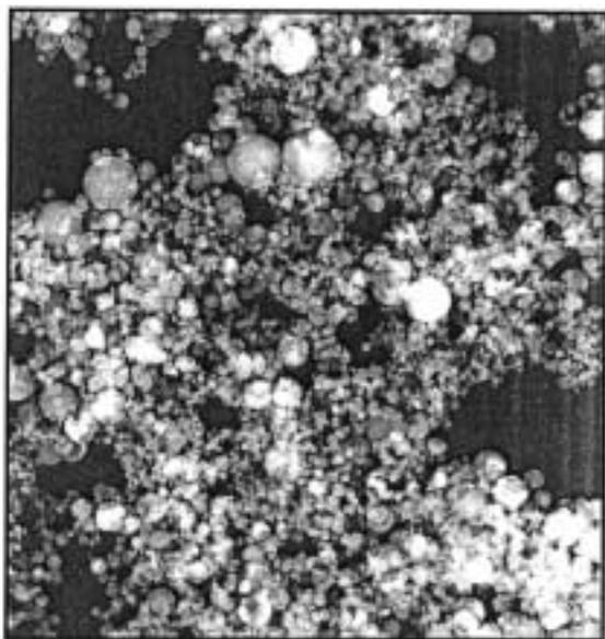
Fig. 1. Typical nano-alumina particle dispersion/morphology from Nanophase Technology Corporation.
