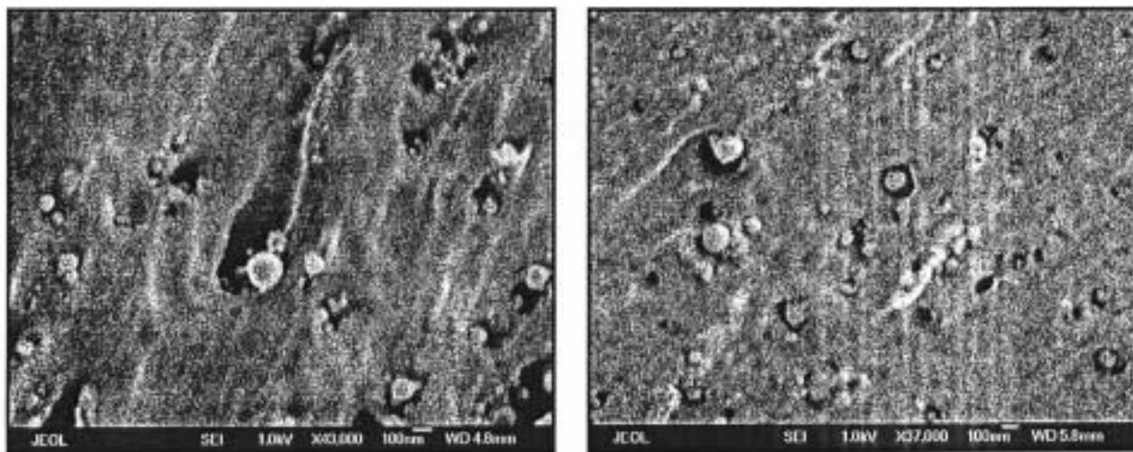
Fig. 8. Yielded composite fracture surface of (left) uncoated nano-alumina particles and (right) silane coated nano-alumina particles at 5 wt% showing good dispersion.
