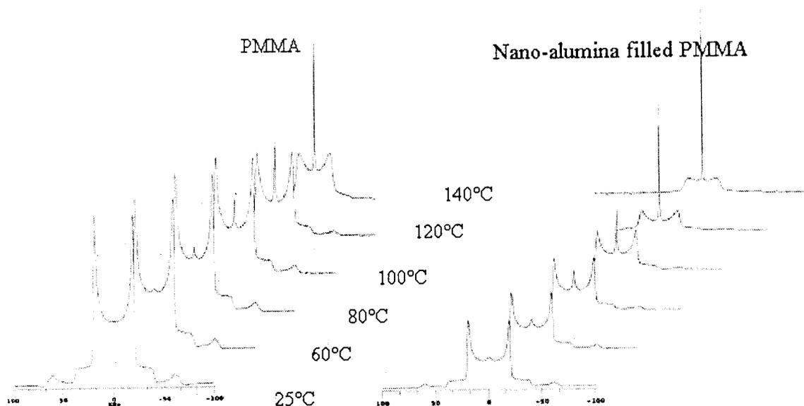
Fig. 9. Representation of data from NMR quadrupolar 1-D experiment with 98% deuterated PMMA during heating runs showing mobility increases. The lowest temperature (25°C) is in the foreground, while the higher temperatures move up and to the right.
