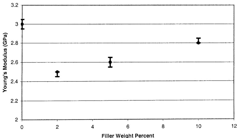
Fig. 5. Young's modulus of nano-alumina filled and neat PMMA as a function of filler weight percent,
