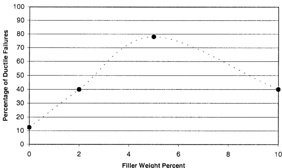
Fig. 4. Percentage of nano-alumina/PMMA composite tensile tests (at  $1 \text{ mm min}^{-1}$ ) resulting in failures past the yield point. The greatest percentage of ductile failures occurred at 5 wt%, where 78% of the failures were ductile in nature.
