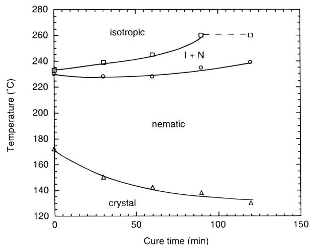
**Figure 2.** Experimentally determined transformation diagram for compound **1** cured at 200 °C. The dotted line indicates those samples that underwent cross-linking before isotropization.
