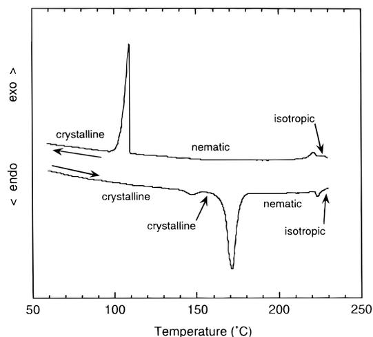
**Figure 3.** DSC heating and cooling curves for compound 1 recorded at 10 °C/min.
