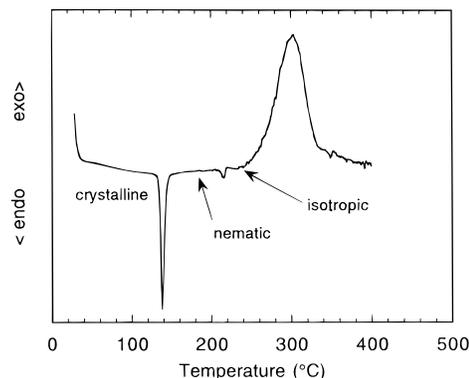
**Figure 4.** DSC heating curve including cross-linking exotherm for compound 9 recorded at 20 °C/min.
