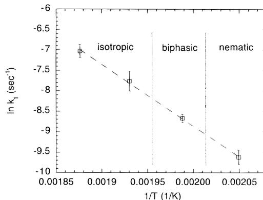
**Figure 6.** Arrhenius plot for the cure of monomer **1** based on the first-order rate constants. Temperature range 215–260 °C. The phase in which the cure takes place at each temperature is also indicated.
