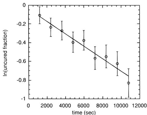
**Figure 5.** First-order kinetic plot for monomer **1** at 215 °C determined by DSC measurements.
