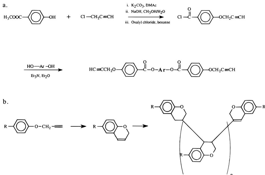
**Figure 1.** (a) Reaction scheme for the synthesis of bispropargyl thermosets and (b) intramolecular propargyl rearrangement followed by chromene polymerization.
