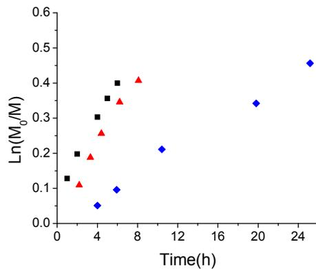
**Fig. 3.** Pseudo first-order kinetic plots for the polymerization of chloroprene with ratio between species [CP]/[RAFT]/[AIBN] = 400: 1: 0.1 with free MDSS (black square); MDSS grafted particles with 0.15 ch/nm<sup>2</sup> density (red triangle); MDSS grafted particles with 0.32 ch/nm<sup>2</sup> density (blue diamond). (For interpretation of the references to color in this figure legend, the reader is referred to the Web version of this article.)
