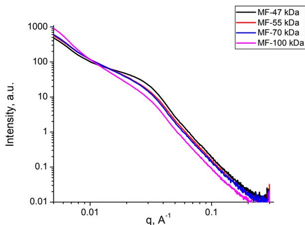
Fig. 5. Representative small-angle X-ray scattering (SAXS) intensity curves for matrix-free PCP grafted silica nanocomposites.
