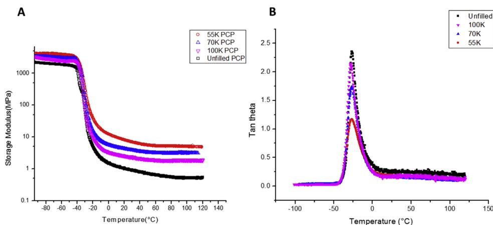
Fig. 7. Temperature dependence of storage modulus of crosslinked unfilled PCP and matrix-free PCP silica nanocomposites.
