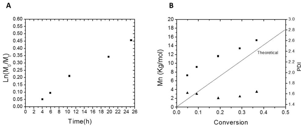
**Fig. 2.** (A) First-order kinetic plot and (b) molecular weight (squares) and polydispersity (triangles) versus conversion of the surfaced initiated RAFT polymerization of CP with 0.32 ch/nm<sup>2</sup> graft density, [CP]/[RAFT]/[AIBN] = 400: 1: 0.1.
