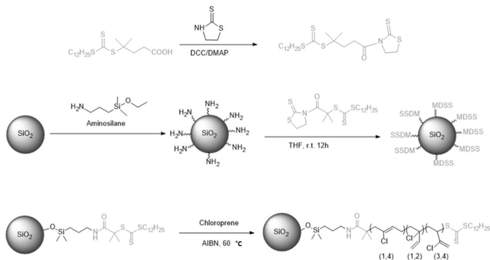
Scheme 1. Preparation of PCP grafted SiO<sub>2</sub> NPs.
