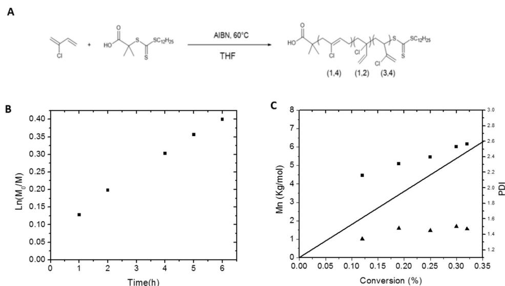
Fig. 1. (A) Reaction scheme, (B) first-order kinetic plot and (C) molecular weight and polydispersity versus conversion for RAFT polymerization of chloroprene in solution.
