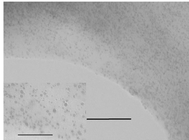
**Fig. 4.** TEM image of 100 kDa PCP grafted silica nanocomposites at 30 silica wt%. Scale bar 500 nm (bottom middle) and 200 nm (bottom left).
