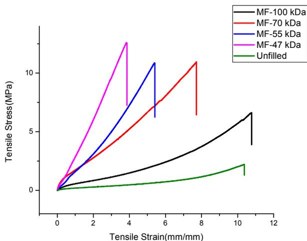
Fig. 6. Stress-strain curves of crosslinked unfilled and filled composites.
