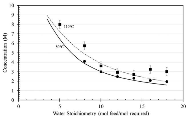
**Figure 4.** Sulfuric-acid concentrations produced in the cell at 0.5 A/cm<sup>2</sup> and either 80 (circles) or 110°C (squares) as a function of water stoichiometry. The water stoichiometry refers to the ratio of the moles of water fed to the cathode to that required via Eqn. 4 at a given current. The lines are the acid concentrations predicted from the Mixed Solvent Electrolyte Thermodynamics Framework (MSE) package in the OLI Systems, Inc. electrolyte software.
