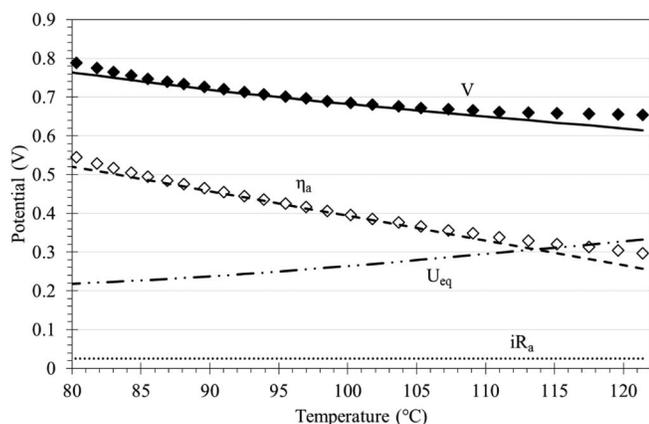
**Figure 6.** Contributions toward total operating voltage across a range of temperatures in the HyS electrolyzer at a current density of  $0.5 \text{ A/cm}^2$  and a constant water flow rate of  $0.50 \text{ mL/min}$ . Lines represent model predictions and the symbols are the cell voltages (filled symbols) and anodic overpotentials (open symbols) data.
