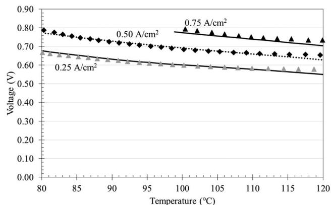
**Figure 7.** Model predictions compared to experimental data at three different current densities across a range of temperatures in the HyS electrolyzer at a constant water flow rate of  $0.50 \text{ mL/min}$ . The solid lines represent model predictions and dotted line represents the model fit at  $0.5 \text{ A/cm}^2$  (i.e., same as the solid line in Fig. 6).
