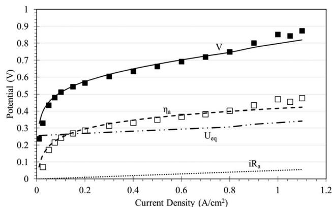
**Figure 5.** Individual potential contributions toward the overall cell voltage for the HyS electrolyzer at 110°C and a constant water feed rate of 0.45 mL/min. Lines represent model predictions and the symbols are the cell voltages (filled symbols) and anodic overpotentials (open symbols) data.
