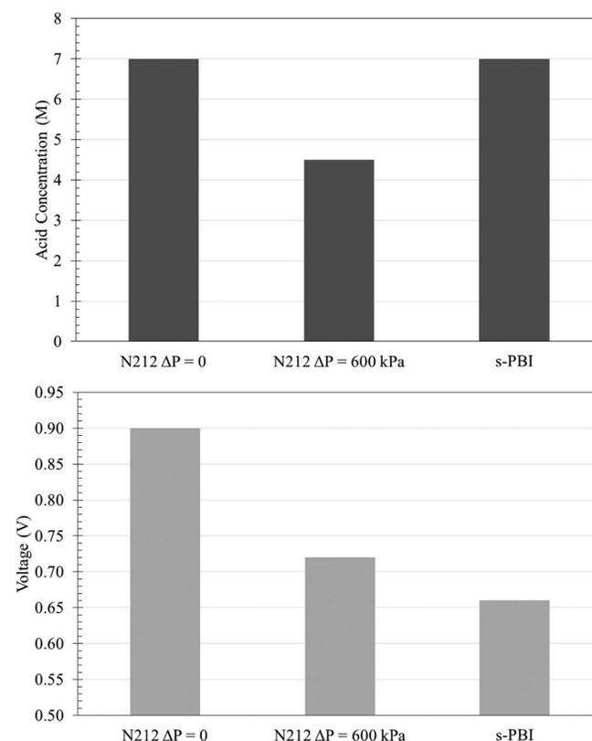
**Figure 1.** a) Sulfuric acid concentration and b) cell voltage at 0.5 A/cm<sup>2</sup> for: Nafion at 80°C and two pressure differentials ( $\Delta P$ );<sup>11</sup> and sulfonated polybenzimidazole (s-PBI) at 110°C.
