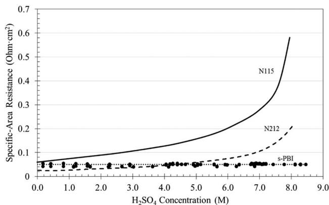
**Figure 3.** Specific area resistance as a function of sulfuric acid concentration for s-PBI obtained from multiple membranes compared to Nafion 115 and Nafion 212.  $\Delta P = 600$  kPa for the Nafion membranes, and no pressure differential used for s-PBI.
