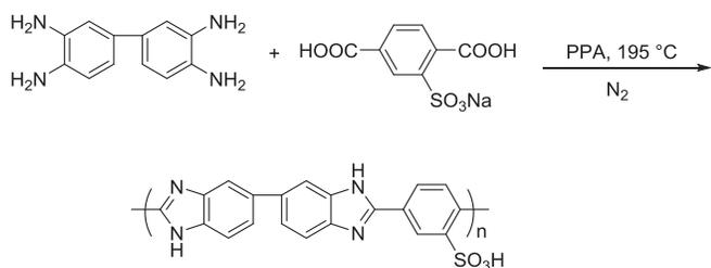
**Figure 2.** Synthesis of s-PBI using mono-sodium-2-sulfoterephthalate and 3,3',4,4'-tetraaminobiphenyl in polyphosphoric acid (PPA).
