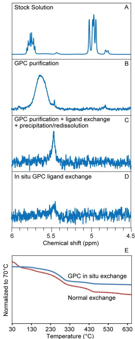
Fig. 4 GPC *in situ* ligand exchange of oleate-capped CdSe QDs with octanethiol. (A–D)  $^1\text{H}$  NMR analysis in toluene, focusing on olefin proton resonances. (A) Prior to ligand exchange. (B) After purification alone. (C) After benchtop ligand exchange performed subsequent to GPC. (D) After *in situ* ligand exchange as indicated. (E) TGA curves of the exchanged NCs prepared by different methods.
