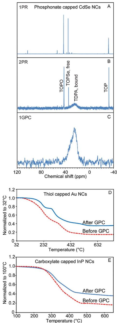
Fig. 1 Purification of NCs with variety of composition and capping ligands. (A)–(C)  $^{31}\text{P}$  NMR of the TDPA-capped CdSe NCs purified by (A) one PR step, (B) two PR steps, and (C) one GPC purification. (D and E) TGA curves for the thiol-capped Au NCs (D) and carboxylate-capped InP NCs (E) before (dashed lines) and after (solid lines) the GPC purification.
