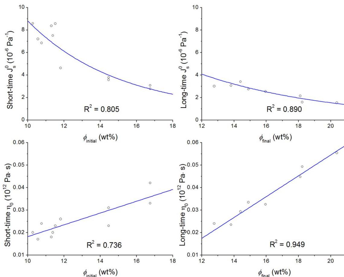
**FIGURE 4** Comparison of the short-time and the long-time values (as defined in the text) of  $J_s^0$  and  $\eta_0$  for para-PBI membranes. The  $J_s^0$  values were fit with exponential functions, and  $\eta_0$  values were fit with lines. Coefficients of regression ( $R^2$ ) are indicated; regression parameters are tabulated in Supporting Information. [Color figure can be viewed in the online issue, which is available at [wileyonlinelibrary.com](http://wileyonlinelibrary.com).]
