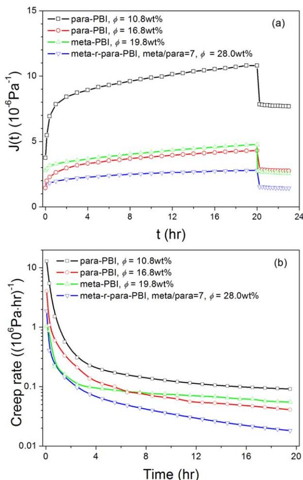
**FIGURE 3** Time-dependent compression creep behavior of selected PBI membranes at 180 °C: (a) creep compliance  $J(t)$  and (b) creep rate  $dJ(t)/dt$ . Indicated solids contents ( $\phi$ ) are values after creep testing. [Color figure can be viewed in the online issue, which is available at [wileyonlinelibrary.com](http://wileyonlinelibrary.com).]
