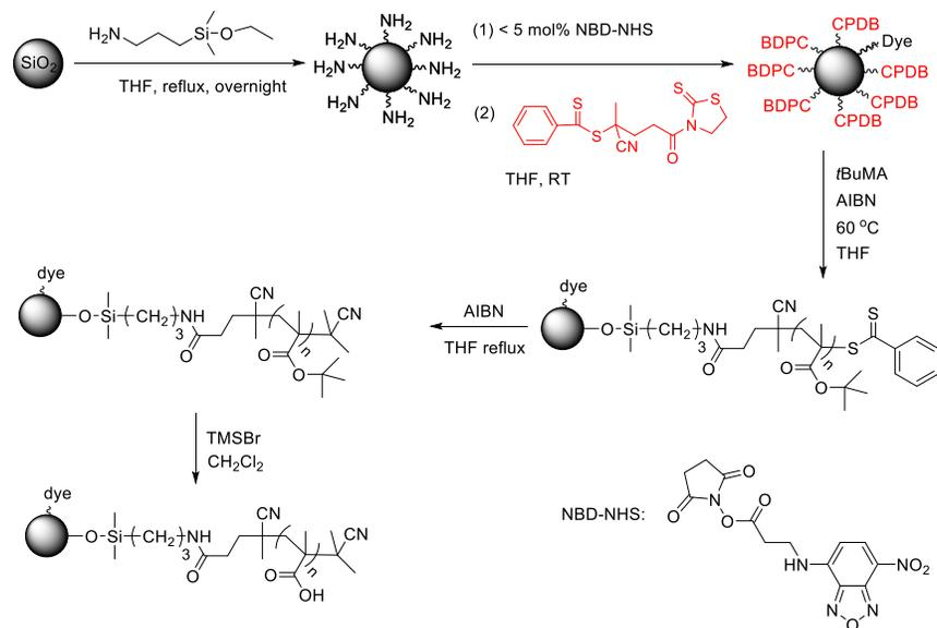
Scheme 1. The synthesis of dye-labeled poly(carboxylic acid) grafted silica nanoparticles. Reproduced with permission from Reference 19. Copyright (2013). American Chemical Society.
