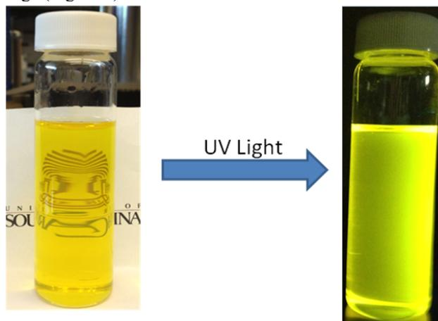
Figure 3. Images of dye-labeled poly(carboxylic acid) grafted silica nanoparticles under UV radiation in DMSO. Reproduced with permission from Reference 19. Copyright (2013). American Chemical Society.
