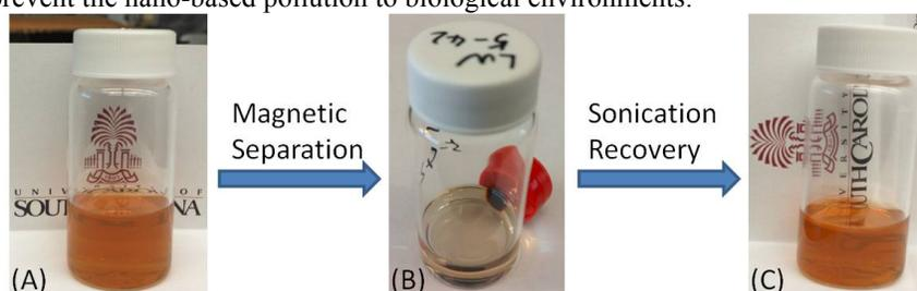
Figure 7. Poly(carboxylic acid) grafted  $\text{SiO}_2/\text{Fe}_3\text{O}_4$  magnetic nanoparticles in dimethylformamide (DMF): (A) Normal state; (B) Under magnetic field; (C) Sonication-recovery and 14 days later. Reproduced with permission from Reference 22. Copyright (2015). Royal Society of Chemistry.
