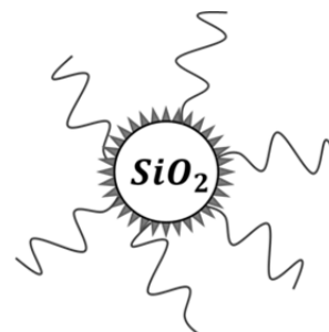
Figure 5. Schematic representation of the bimodal brush grafted core functionalized silica nanoparticle. The short brush is oligothiophene and long brush is PGMA.
