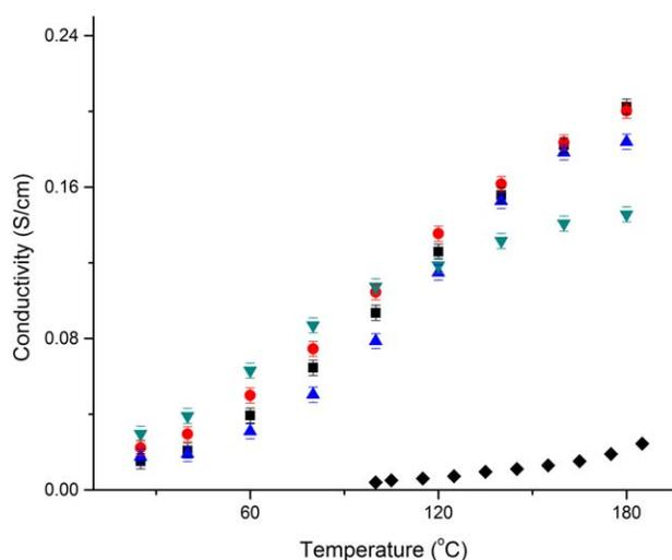
**FIGURE 5** Anhydrous conductivity evaluation for *r*-AB-PBI at 180 °C [squares: *i*-AB-PBI, circles: 70:30 *i*-AB:AB, triangles: 50:50 *i*-AB:AB, inverted triangle: 30:70 *i*-AB:AB, diamonds: reported literature values for poly(2,5-benzimidazole)(AB-PBI)<sup>60</sup>]. [Color figure can be viewed in the online issue, which is available at wileyonlinelibrary.com.]
