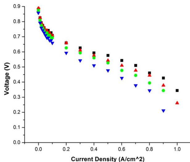
**FIGURE 9** Polarization curves for *i*-AB-PBI using H<sub>2</sub>:Air 1.2:2.0 stoichiometric flows, respectively [squares: 180 °C, triangles: 160 °C, circles: 140 °C, inverted triangles: 120 °C]. [Color figure can be viewed in the online issue, which is available at [wileyonlinelibrary.com](http://wileyonlinelibrary.com).]
