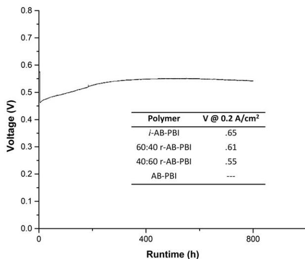
**FIGURE 10** Lifetime fuel cell performance of 40:60 (*i*-AB:AB) r-AB-PBI membrane. Inset: fuel cell performance observed over compositional range for the r-AB-PBI copolymer system. Data collected from fuel cells operated at 180 °C supplied with hydrogen/air at 1.2:2.0 stoichiometric flows, respectively, under 1 atm without applied backpressure or humidification.
