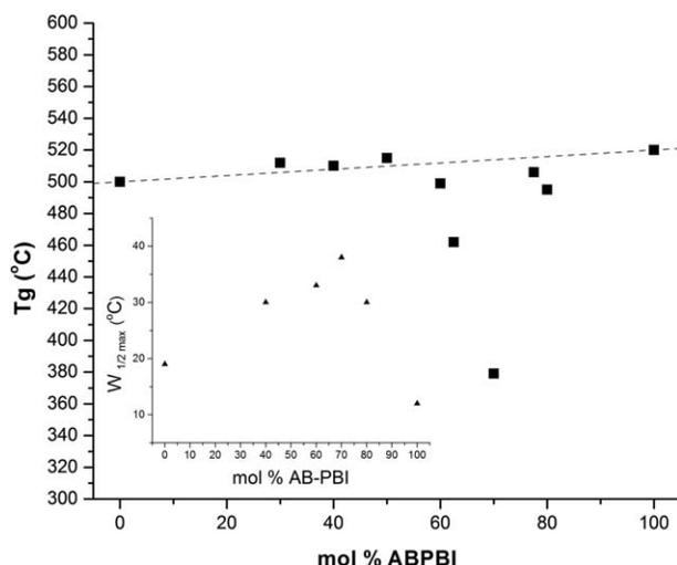
**FIGURE 4** Effect of copolymer composition on glass transition temperature,  $T_g$ . Repeat measurements were conducted and error of  $\pm 1$  °C was determined. Dashed line is a calculated plot of the Fox equation. Inset: plot of  $\tan \delta$  peak width at half max with respect to composition.
