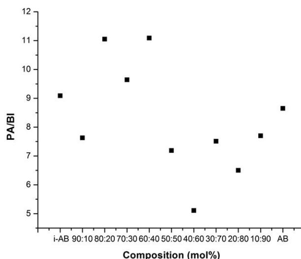
**FIGURE 6** Variation of acid loading with copolymer composition for *r*-AB-PBI copolymers. PA/BI: moles PA per mole of benzimidazole.
