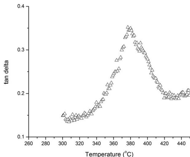
**FIGURE 3** DMA  $\tan \delta$  plot of r-AB-PBI (30:70 *i*-AB:AB).
