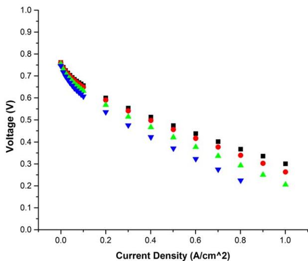
**FIGURE 8** Polarization curves for 60:40 *i*-AB-PBI:AB-PBI using H<sub>2</sub>:Air 1.2:2.0 stoichiometric flows, respectively [squares: 180 °C, circles: 160 °C, triangles: 140 °C, inverted triangles: 120 °C]. [Color figure can be viewed in the online issue, which is available at [wileyonlinelibrary.com](http://wileyonlinelibrary.com).]
