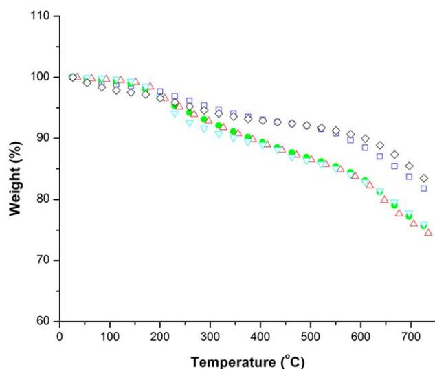
**FIGURE 2** Thermal gravimetric analysis. Squares: *i*-AB-PBI, dot: 70:30 *i*-AB:AB, upward triangle: 50:50 *i*-AB:AB, downward triangle: 30:70 *i*-AB:AB, diamond: AB-PBI. [Color figure can be viewed in the online issue, which is available at wileyonlinelibrary.com.]
