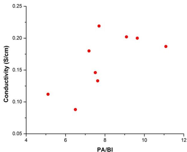
**FIGURE 7** Effect of phosphoric acid loading on ionic conductivity at 180 °C for r-AB-PBI copolymers. PA/BI: moles PA per mole of benzimidazole. [Color figure can be viewed in the online issue, which is available at [wileyonlinelibrary.com](http://wileyonlinelibrary.com).]
