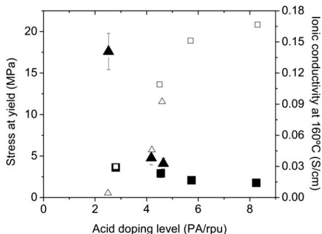
**FIGURE 6** Effect of acid doping level on stress at yield (filled) and ionic conductivity at 160 °C (unfilled) for heat-treated conventionally imbibed ( $\blacktriangle$  and  $\Delta$ ) and sol-gel ( $\blacksquare$  and  $\square$ ) PA-doped *m*-PBI membranes.
