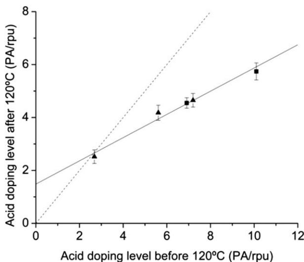
**FIGURE 2** Acid doping level before and after heat treatment for sol-gel PA-doped *m*-PBI membranes (-■-) and conventionally imbibed membranes (-▲-). The dashed line indicates the line expected for no PA loss during heat treatment, and the solid line is the fitted line (linear regression) for the data.
