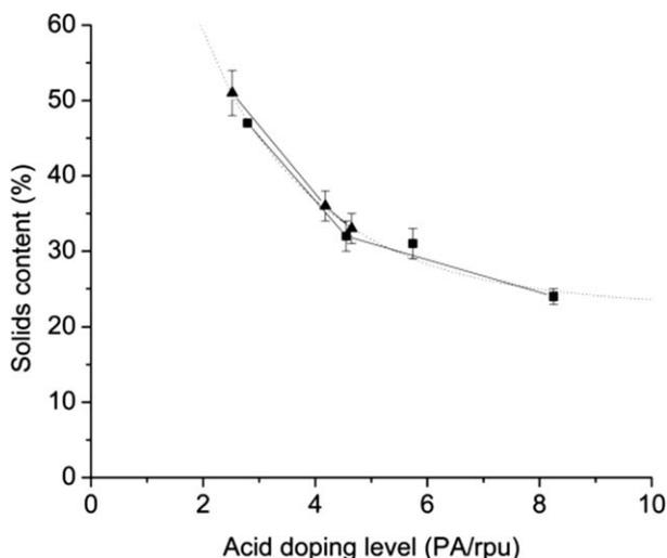
**FIGURE 1** Correlation of solids content and acid doping level for heat-treated PA-doped *m*-PBI membranes for PA-doped *m*-PBI membranes prepared by the sol-gel process (-■-), conventional imbibing (-▲-), and exponential fit ( $y = 0.2 + 0.9 e^{-x/2.2}$ ) of the data (---).
