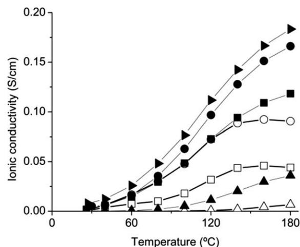
**FIGURE 4** Ionic conductivities for heat-treated PA-doped *m*-PBI membranes at different acid doping levels for conventionally imbibed membranes [ $3 \pm 0.3$  (▲),  $4 \pm 0.3$  (□), and  $5 \pm 0.3$  PA/rpu (○)] and sol-gel membranes [ $3 \pm 0.2$  (▲),  $5 \pm 0.2$  (■),  $6 \pm 0.3$  (●), and  $8 \pm 0.7$  PA/rpu (▶)].
