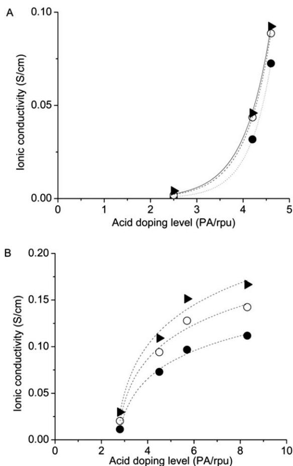
**FIGURE 3** Effect of acid doping level on ionic conductivity for heat-treated (A) conventionally imbibed and (B) sol-gel *m*-PBI membranes at 120 °C (●), 140 °C (○), and 160 °C (▲). The error in acid doping level was  $\leq 0.3$  PA/rpu, except for the highest acid doping levels ( $8 \pm 0.7$  PA/rpu).
