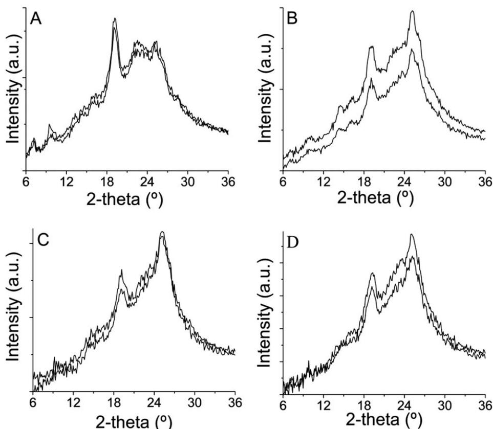
**FIGURE 7** WAXS spectra of heat-treated (A and C) conventional ( $5 \pm 0.3$  PA/rpu and  $33 \pm 2$  wt % solids) and (B and D) sol-gel ( $5 \pm 0.2$  PA/rpu and  $32 \pm 2$  wt % solids) PA-doped *m*-PBI membranes. A and B are one-dimensional WAXS scans in reflection geometry taken parallel and perpendicular to the cast direction. C and D are one-dimensional WAXS scans in transmission geometry taken parallel and perpendicular to the cast direction.
