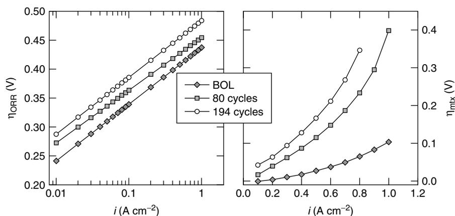
**Figure 7.** ORR and mass-transport overpotential development as function of cycle number in a voltage cycling test (cycling between 0.6 and 0.85 V, 180 °C) calculated as described in Ref. [39]. [Reproduced from Ref. [39] © Elsevier, 2008.]
