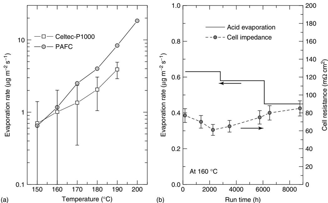
**Figure 6.** (a) Phosphoric acid evaporation rates in Celtec<sup>®</sup> MEAs at the beginning of life as function of temperature. For comparison, PAFC data from the literature are included. PAFC data are extracted from Okae and coworkers.<sup>[38]</sup> (b) Phosphoric acid evaporation rate in Celtec<sup>®</sup> MEA operated at  $160^{\circ}\text{C}$  over a period of one year (left axis) and the cell resistances measured by 1-kHz AC impedance spectroscopy (right axis).
