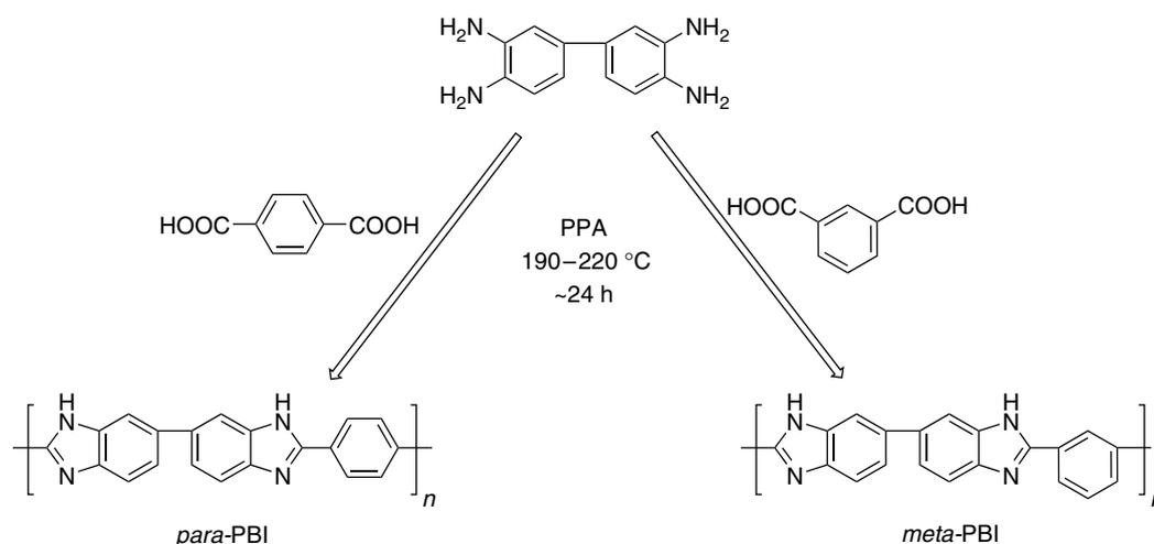
**Scheme 1.** General synthetic scheme for the synthesis of PBI in PPA (polyphosphoric acid).
