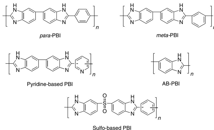
**Scheme 2.** Examples of polybenzimidazole (PBI) chemistries prepared through the polyphosphoric acid (PPA) process.
