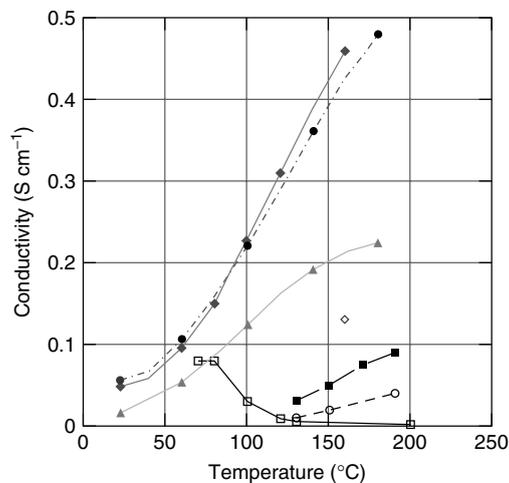
**Figure 2.** Through-plane conductivity–temperature behavior for several PEMs (□ Nafion, ■ PBI cast from trifluoroacetic acid, ◇ *m*-PBI cast from DMAc (conventional membrane preparation),<sup>[9]</sup> ○ PBI from conventional DMAc casting method, ● ◆ ▲ *p*-PBI chemistries prepared via the PPA process). All membranes were prepared in the Benicewicz research group at Rensselaer Polytechnic Institute. [Reproduced from Ref. [9] © Springer, 2001.]
