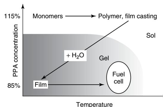
**Figure 1.** State diagram of the PPA sol–gel preparation process.
